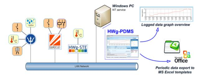
**Note:** PDMS supports converting pulses coming from energy meters to kWh or liters.
