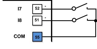
Driving an input against the supply voltage
